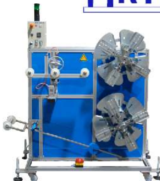
twin-station winder with mechanical laying unit and dancer control
