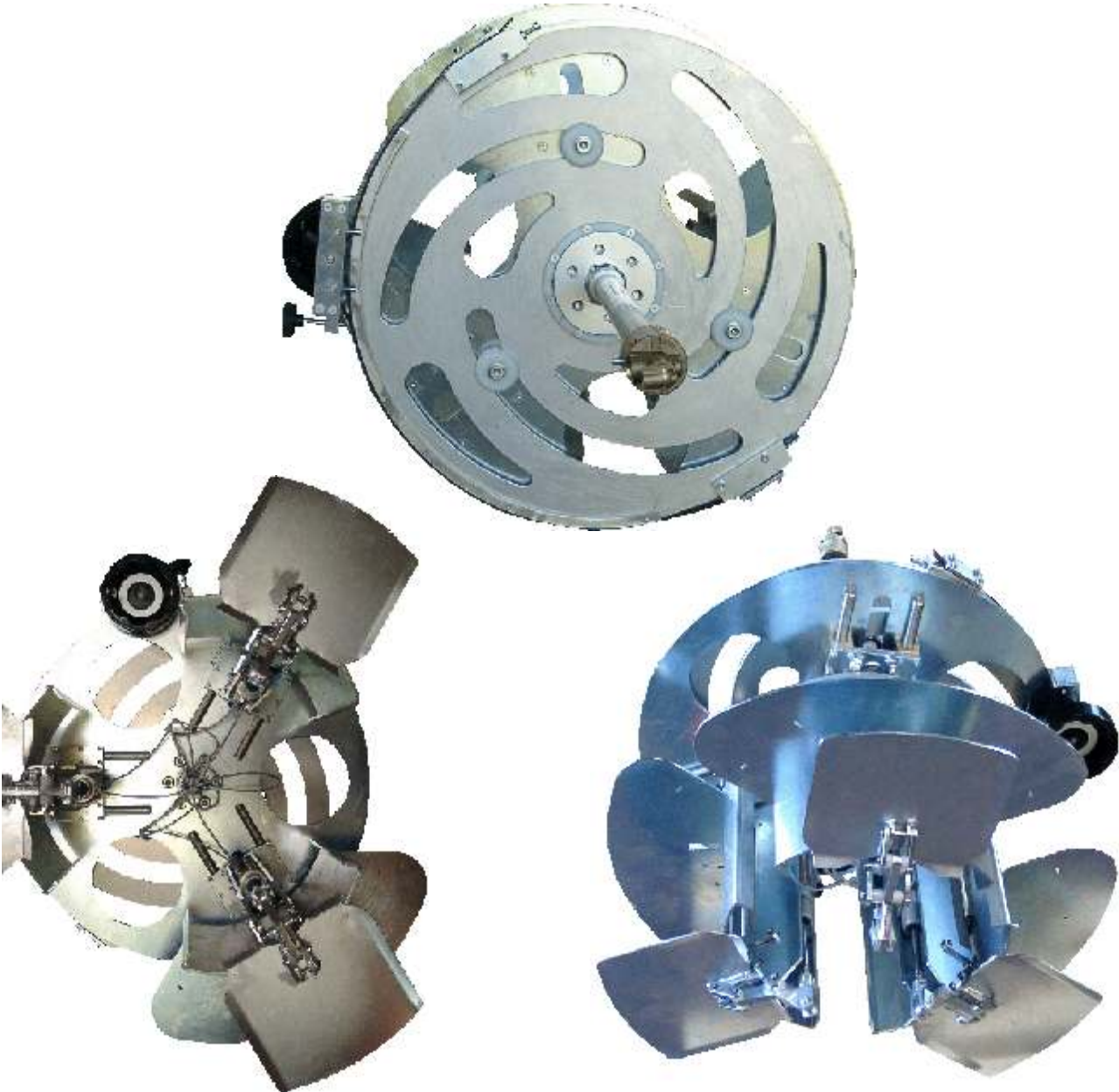
manual collapsible reel with variable width and adjustable core diameter
