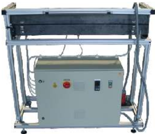
heating tunnel with infrared heaters
