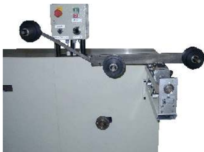
single-station winder with mechanical laying unit
