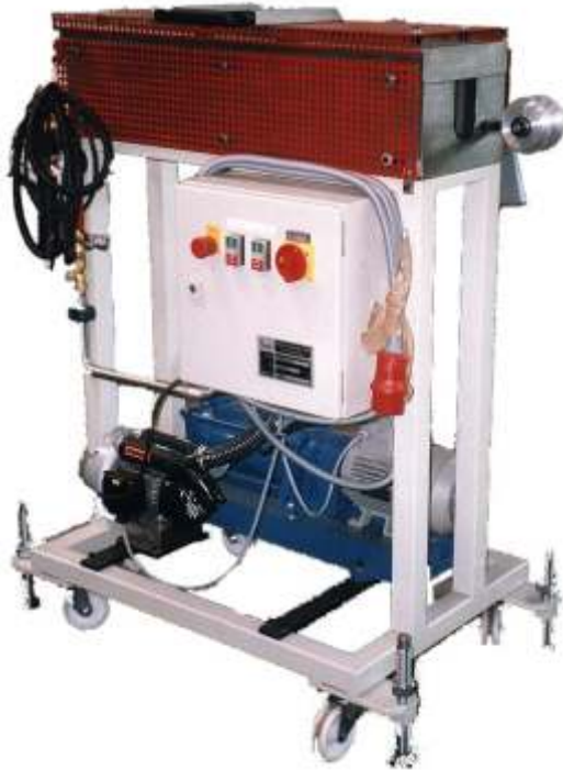
warm air heating tunnel
