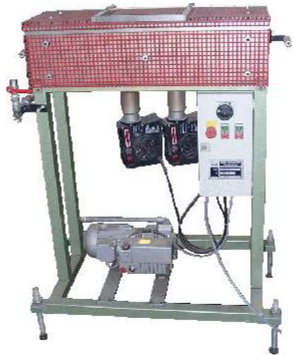
warm air heating tunnel
