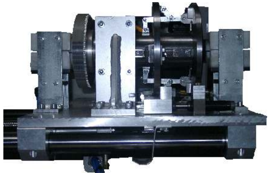
cutter for splinter free cutting of thin-walled pipes
