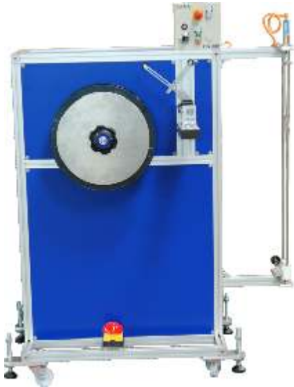
single-station winder with mechanical laying unit and dancer control
